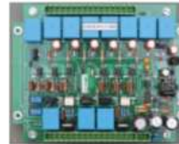
'All in One PLC card' for Mechanical Loom
