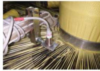
"Weft Break Detection" for avoiding Fabric Wastage
