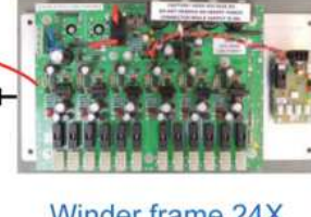
Winder frame 24X 'Synchronizer' Power Supply card Auto & Manual Avoids Total Frame Failure
