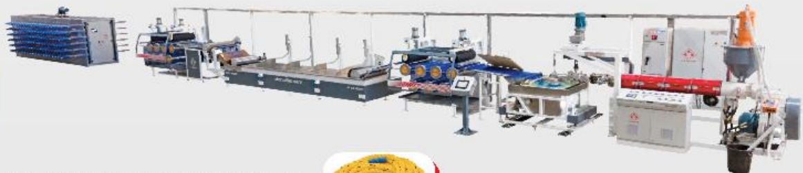
PE/PP MONOFILAMENT LINE WITH COP WINDERS /DUNLINE PLANT
