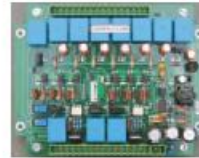
"Weft Break Detection" for avoiding Fabric Wastage
