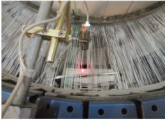
"Weft End Detection" for reducing tape wastage
