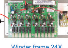
Winder frame 24X Power Supply card
