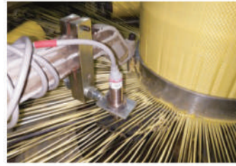
"Weft Break Detection" for avoiding Fabric Wastage
